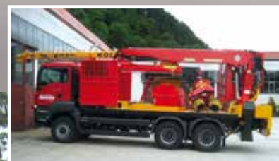
K307GH 4-axe truck for up and downhill logging
