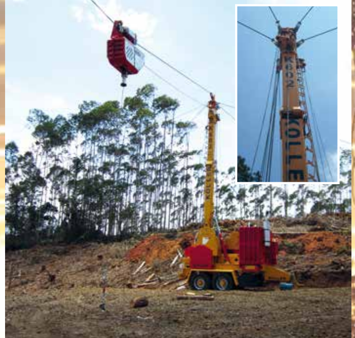
K602H with hydraulically foldable tower
