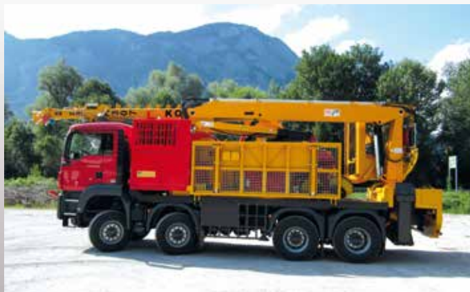
K307GH 4-axe truck for up and downhill logging
