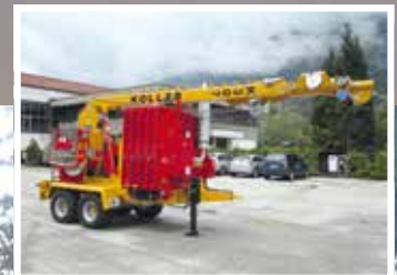
K307H with hydraulically foldable tower
