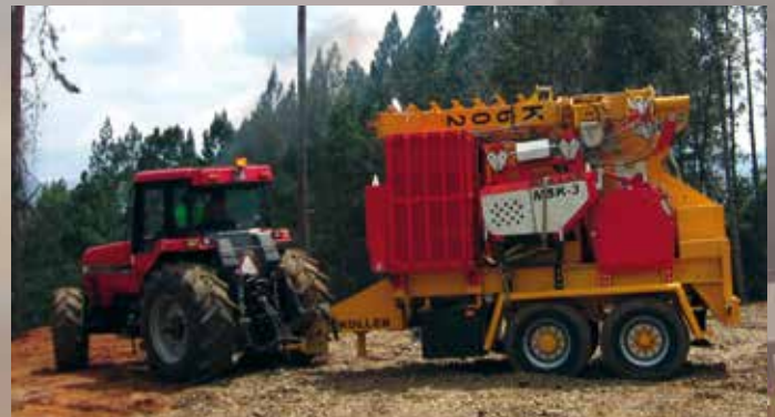
K602H with hydraulically foldable tower
