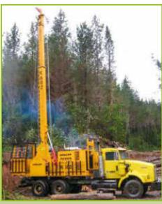
The **K 602-A** is a powerful yarder for uphill logging. The machine is equipped with a self-supporting frame, allowing a simple assembly on various trucks or trailers as well as easy worldwide export. It is principally used for selective cuts and for general wood harvesting operations.
